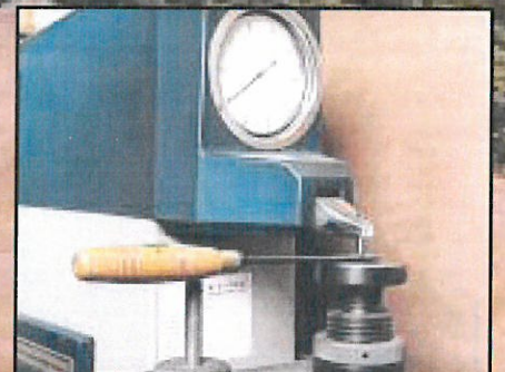
Testing the finished blade for hardness.
