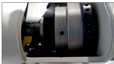
36-position indexing on spindle
