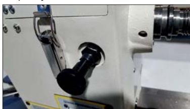
indexing pin and quick release of pulley cover
